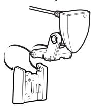
3. Put the pivot bolt through the assembly to hold it in position and loosely install the nut, but do NOT tighten the nut at this time. Insert the pivot arm assembly into the mounting bracket. Do NOT snap the assembly closed, as you will need to access the mounting bracket in the next step.
